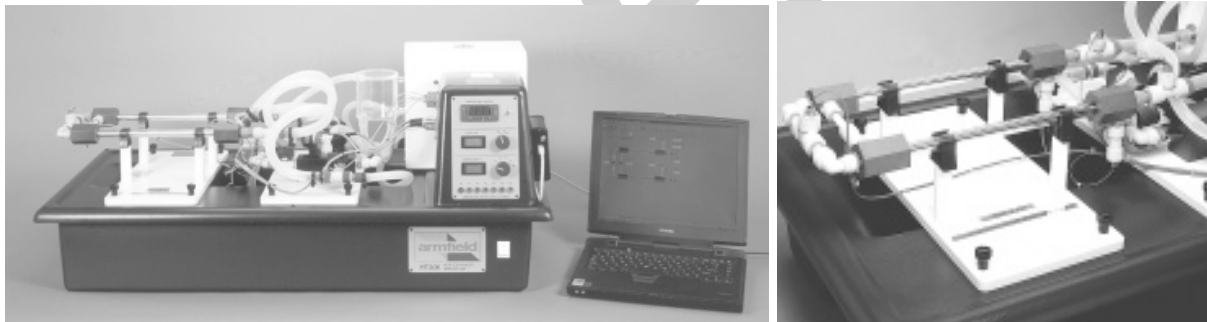
Σχήμα 2. ARMFIELD – Heat Exchanger Teaching Equipment. HT30X service unit (μονάδα εξυπηρέτησης) with the HT31 Tubular Heat Exchanger
